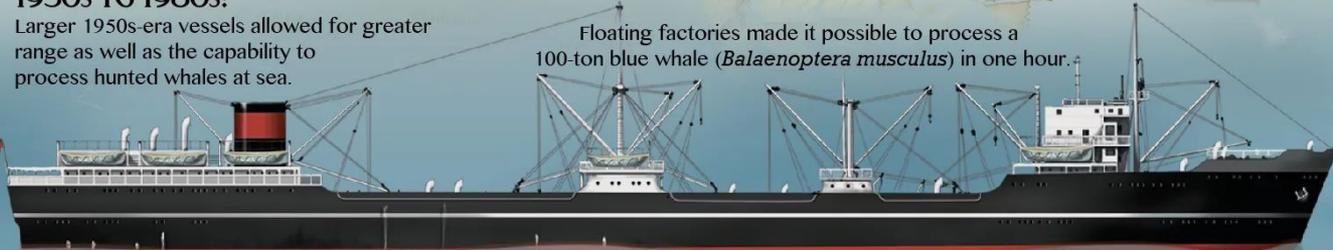
Carcasses were winched up onto an open butchering deck via a slipway through the stern.
